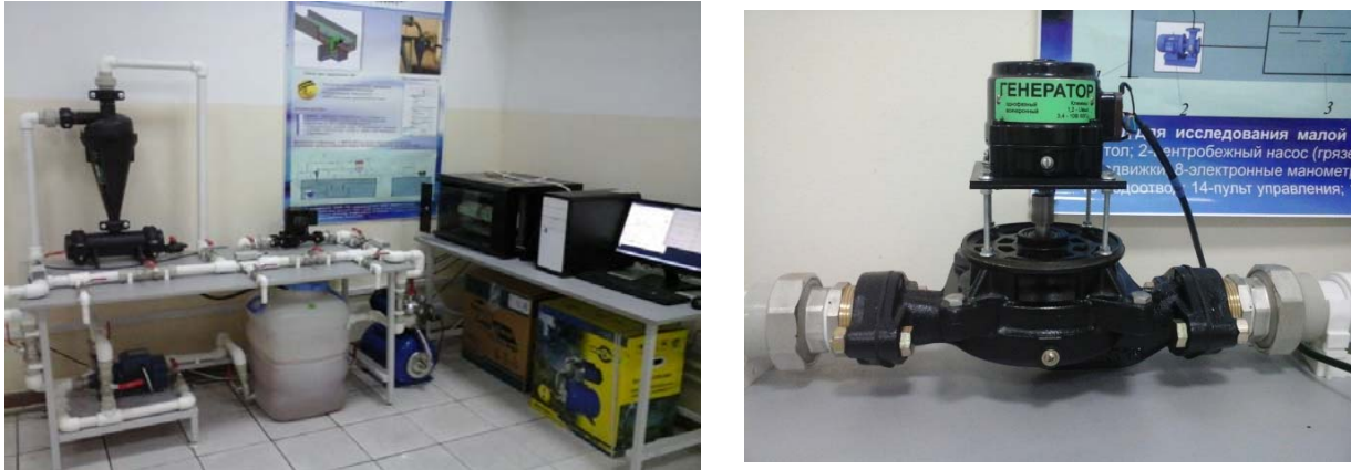
Figure 5 – Laboratory stand (a) and a hydraulic turbine with a generator (c)
