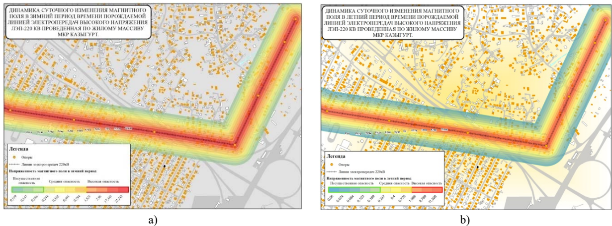
Figure 6 – GIS map describing the dynamics of changes in the magnetic field in 220 kV high-voltage power lines in the summer (a) and winter (b) periods of time in the residential area of the Kazygurt microdistrict
