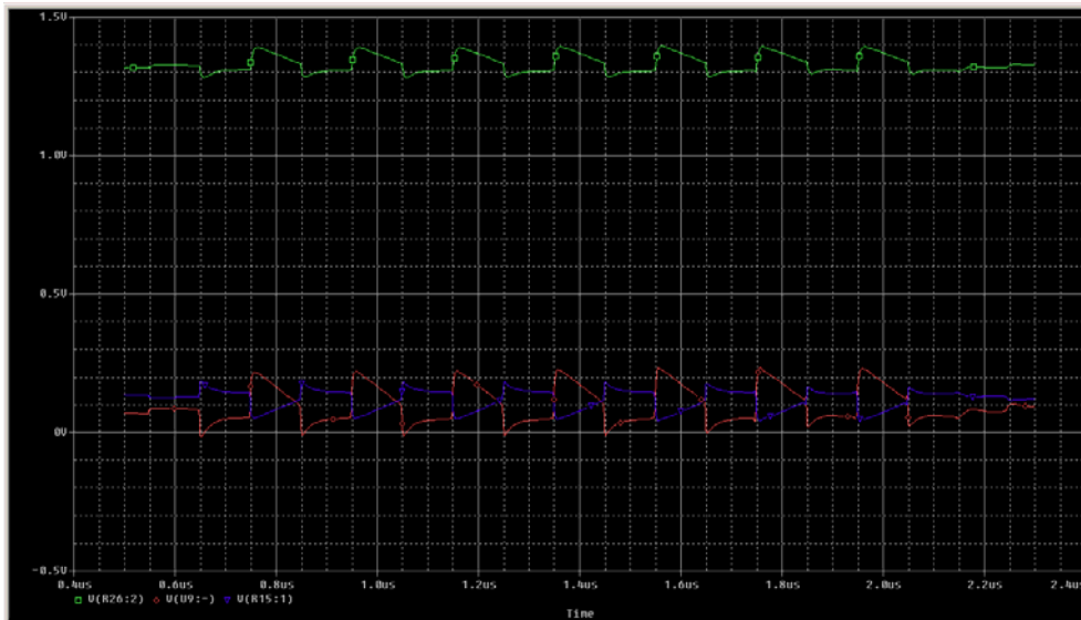
Figure 8 – Diagrams of antiphase signals U(U 9 ; N) and U(R 15 ; 1) at the output of a long line of and output signal U(R 2 ; 2) at 100 Mbit/s on the same scale
