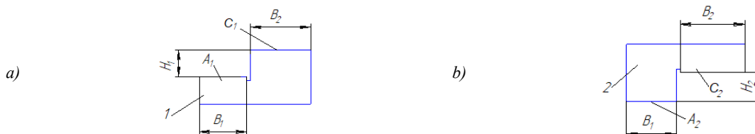
Figure 3 – Layouts of the dimensions of the combined surfaces of parts. a - part 1; b - part 2
